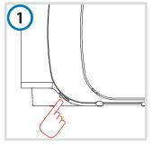
Switch the machine off by pressing the power on/off switch.
