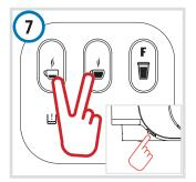
Press and hold the **espresso** and **long coffee** buttons simultaneously and at the same time turn on the machine by pressing the power on / off switch.
