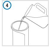
Mix the contents of a bottle of Caffitaly System descaling agent with approximately 750 cc. of water (a total of 1 litre) and pour into the tank.
