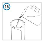
Carefully empty and rinse out the water tank and refill it with fresh, still water.
