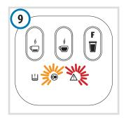
The appliance dispenses the descaling agent at intervals (5 doses with a 4 minute pause between each one, for a total duration of about 25 minutes). During this step, when the buttons must not be pressed, the *descaling* and *multifunction* warning lights blink respectively in YELLOW and RED alternately. If the container fills up, empty it
