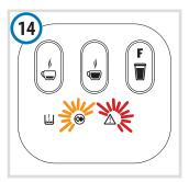
Rinse water (about 500 ml) will be run through the machine. During this stage, the *descaling* and *multifunction* warning lights blink alternately.
