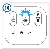
When the first step is over, the **long coffee** button lights up and the machine beeps repeatedly. The water tank is empty.
